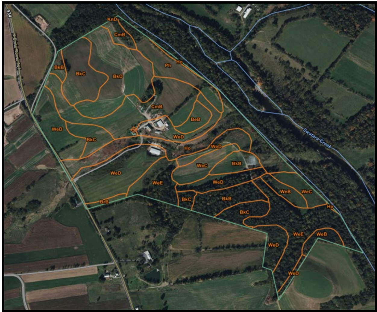
Figure 23. Soils map shows that the project is to fall in a BuB (Bucks silt loam) soil zone. If advised it may be feasible to move the arrays to the RaB zone east of the buildings.
